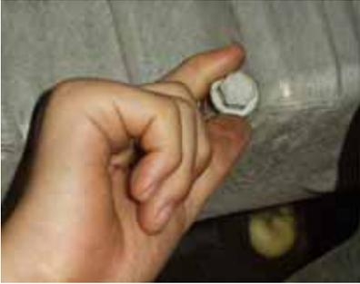
Drain the oil. There have been discussions whether through-the-dipstick oil removal, as used on other Mercedes engines, works. I jerry rigged a system to test it out – I was not successful. It left 1.5 qts behind.
