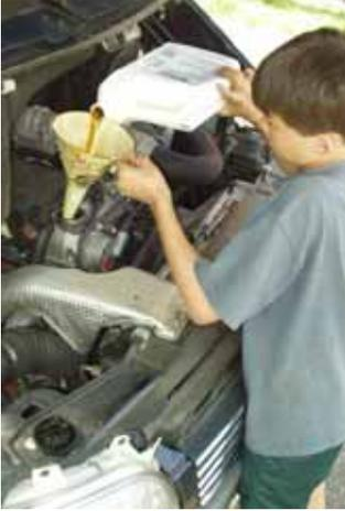
Reinstall the oil drain plug. Reinstall and hand tighten the oil filter cap. Then refill crankcase with 9.5 quarts of approved oil. Don't forget to reinstall the oil filler cap.
