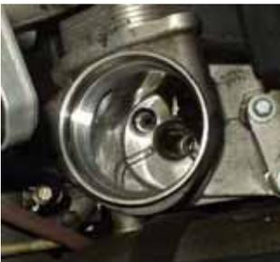
There have been several discussions as to whether there is a mess in pulling the filter from the block-integral oil filter canister. That is not the case. The oil drains directly into the block. Note the condition of the canister upon removal of the filter.
