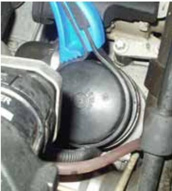
Loosen and remove the oil filter cap.
