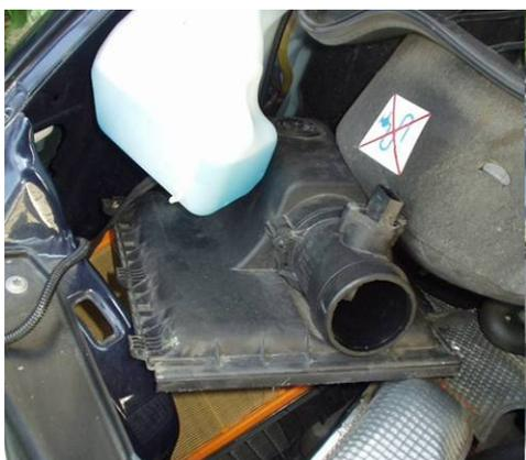
The trick: Wiggle the top around so that the hump is between the windshield washer and the interior fan casing, and bring the flanges up over the heat shield and headlight frame. The picture shows the angle to aim for. Slide out the top.
