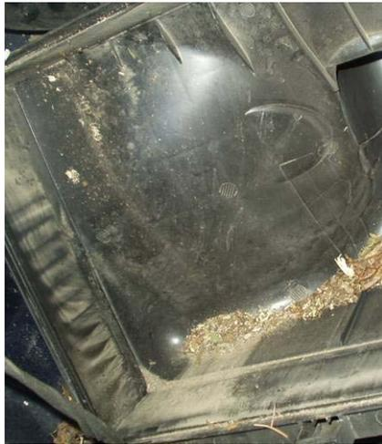
Clean out the supply side of the air filter housing. I found a shop vacuum was the quickest.
